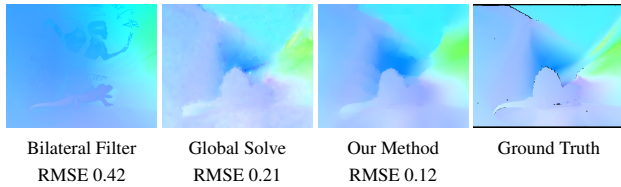
Figure 7: A comparison of different methods for propagating sparse correspondences to compute optical flow. The results shown here were generated using each authors' publicly available code, and choosing parameters that yielded the lowest RMSE between ground truth and estimated flow vectors (in pixels).
